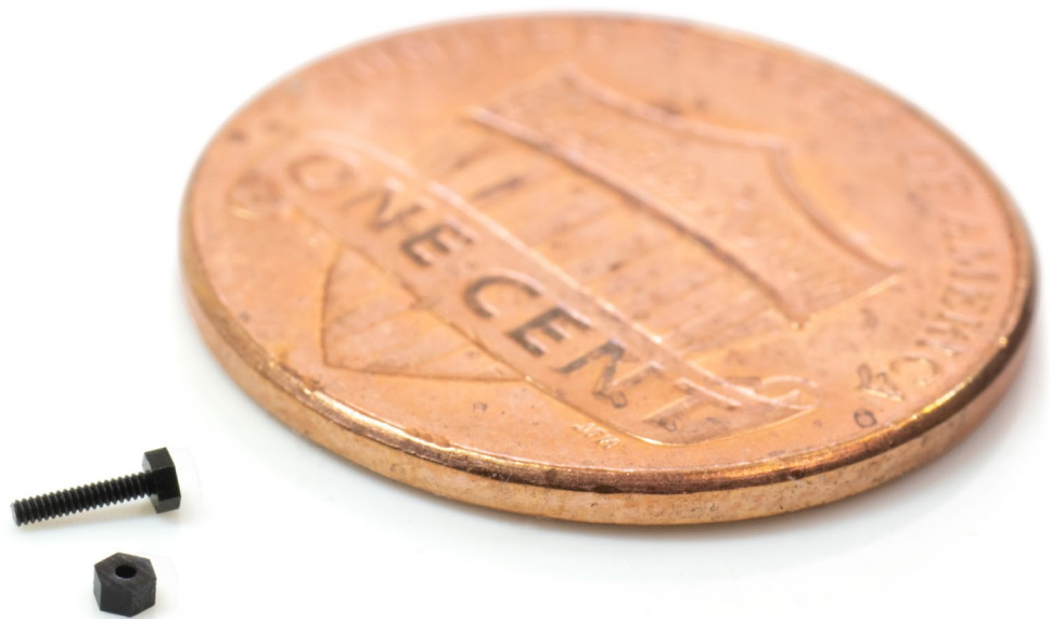
Figure 1: A 3D printed micro nut and bolt with M0.3 threads
